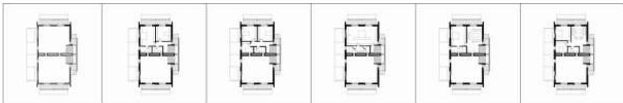
**Figure 5:** The static plan on the left can be transformed to the following plans by the occupants.
